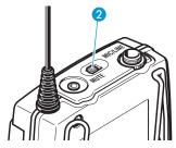
The MUTE switch 2 allows you to mute the audio signal or to deactivate the RF signal.
