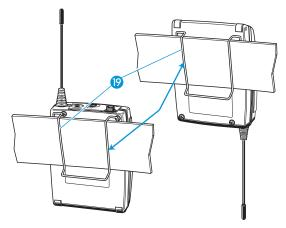
The belt clip is detachable so that you can also attach the bodypack transmitter with the antenna pointing downwards. To do so, withdraw the belt clip from its fixing points and attach it the other way round.
