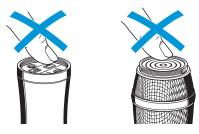
When unscrewing the microphone head **1** during operation, the muting function is automatically activated. "MUTE" appears on the display panel.
