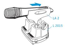
Plug the LA 2 charging adapter with the inserted radio microphone into the L 2015 charger (see "Accessories and spare parts" on page 30).
