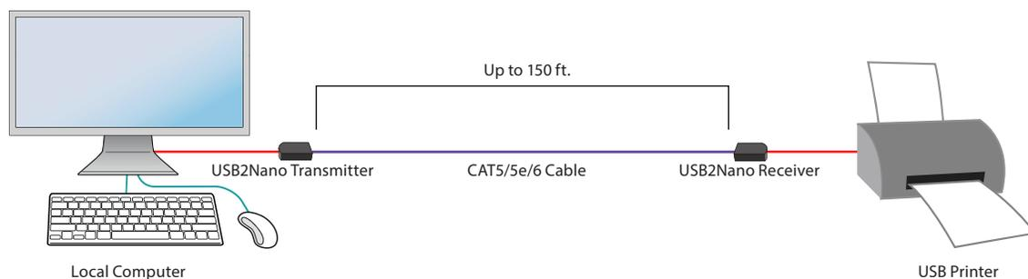
Any USB 2.0 Device can be connected
