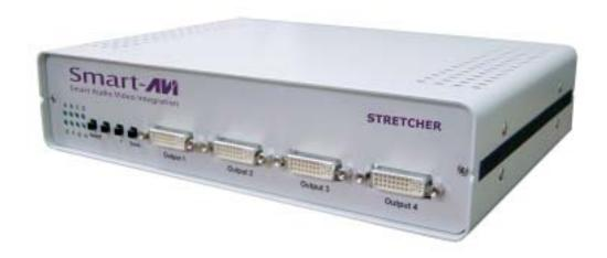
The SmartAVI UXST4 is a display wall controller which connects to the VGA output of any PC and displays the image across 4 displays. Each display shows 1/4 of the VGA image in a 2 x 2 format.
