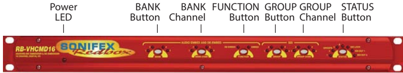
Fig 5-2: RB-VHCMD16 Front Panel
