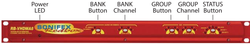
Fig 2-2: RB-VHDM8 Front Panel
