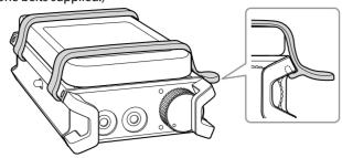
• If the audio device does not mount on the rubber rails of the unit, insert the protection sheet (supplied) between this unit and the audio device, to reduce
