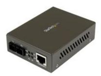
The MCMGBSC055 1000 Mbps Gigabit Multi Mode Fiber Ethernet Media Converter SC - 550m converts transparently to/from 1000Base-T Ethernet signals and 1000Base-SX optical signals, providing a cost-effective Ethernet-fiber/copper-fiber link, in order to extend an Ethernet network connection over a Multimode fiber backbone.
