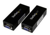
The ST121UTPEP VGA Video Extender over Cat5 - Point to Point lets you connect a remote VGA display/projector up to 80m (250ft) away from the VGA signal source. The ST121UTPEP is a bundled kit that includes both a local and a remote unit providing a complete end to end solution for a single source/display connection, transmitting the source VGA signal over a standard Ethernet cable (Cat5e or better UTP cable, terminated with RJ45 connectors).
