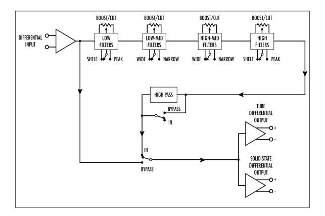
The electronically balanced input stage input goes directly into the passive EQ sections. The low and high bands can switch between peaking and shelving filters, the low mid and high mid can switch between narrow and wide bandwidths.
