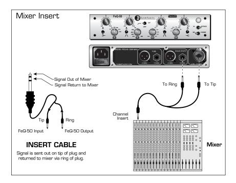
**Note:** Check the Insert level on your mixer. If your mixer uses a Odb to +4dB insert point, use the +4dB input and output on the FeQ-5O and an insert cable with XLR connectors.
