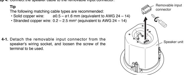
**4-2.** Insert the stripped cable end into the terminal and tighten the terminal screw with a screwdriver.
