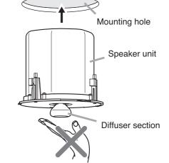
Rotate and tighten the mounting tab axis screws (3 places) on the unit clockwise to their full stop in order to grip the ceiling panel with the mounting tabs.
