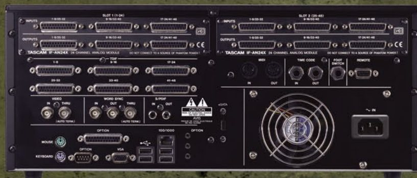
Pictured with optional IF-AN24X analog interface cards installed
