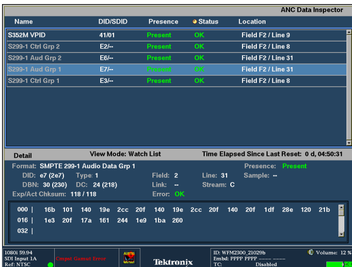
ANC Data Inspector provides detailed content analysis.
