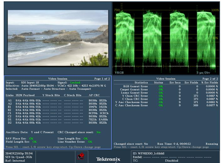
The FlexVu™ four-tile display provides maximum flexibility to increase your productivity. Unlike instruments with predetermined view combinations or limited choices, FlexVu™ lets you create a multiview display tailored to your specific needs and work practices. Each tile can be configured to enable easy signal analysis such as multiple alarm and status screens, different Safe Area Graticules and cursors on each tile, and more.
