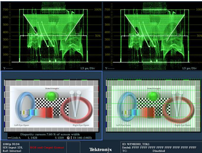
For measurement of the depth of an object within the image a Disparity Grid can be overlaid over the picture with a horizontal disparity between 1 to 15% of screen width and a vertical disparity of 50%, 25%, or 10% that can be selected by the user. The horizontal and vertical position controls allow the Disparity Grid to be moved around within the picture display to gauge the depth of objects within the image.
