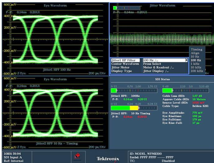
With FlexVu™, users can simultaneously display timing jitter and alignment jitter values, cable parameter measurements, and display different eye patterns to help quickly diagnose and resolve problems related to SDI timing jitter or cable attenuation. The infinite persistence mode of the waveform monitor can also be used to more easily view the eye opening of the physical-layer signal.
