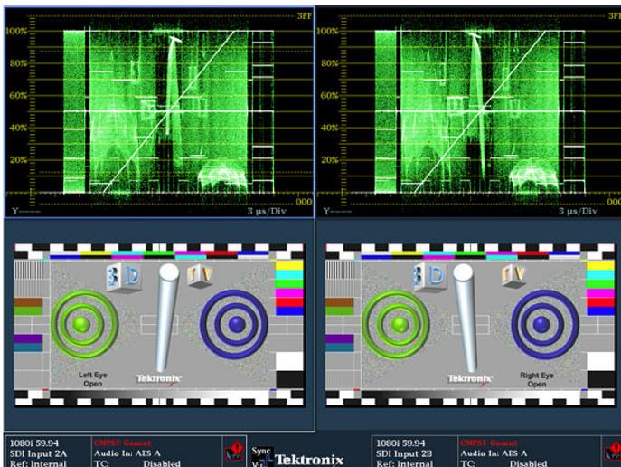
FlexVu™ enables flexible and intuitive configuration of displays from two monitored inputs. User can display simultaneous fault detection, status reporting, alarm generation, and error logging. SIM is ideal for transmission monitoring of simultaneous HD and SD programs. It is also ideal for monitoring stereoscopic 3D content in production and post production applications by simultaneously monitoring the Left Eye signal and the Right Eye signal.
