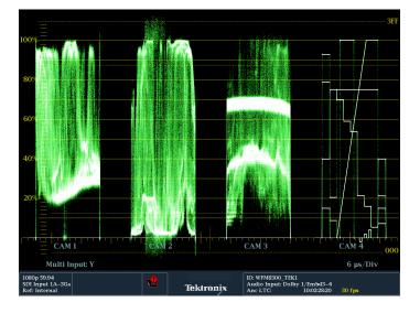
Multiple Input mode can be used to monitor up to 4 SDI inputs simultaneously when in Full Screen mode (4-input mode requires Option 2SDI). This type of display is ideal for camera balance applications where the user wishes to check the video level across multiple inputs. This Multiple Input mode is available within Waveform, Vector, Lightning, Diamond, Arrowhead, and Spearhead (with Option PROD) display modes, allowing for the comparison of video inputs across a wide variety of these displays.
