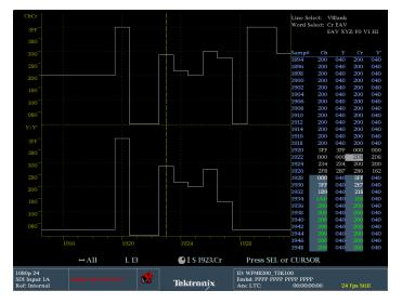
The Datalist display, available as standard on the WFM8300 and available as part of Option DAT on the WFM8200, provides detailed information on the actual data values in HD/SD-SDI and 3G-SDI (with Option 3G) input signals. Users can easily use this display to locate protocol errors in the input signals.
