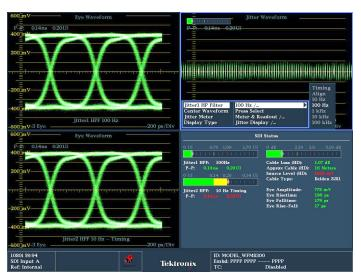
With FlexVu<sup>™</sup>, users can simultaneously display timing jitter and alignment jitter values, cable parameter measurements, and display different eye patterns to help quickly diagnose and resolve problems related to SDI timing jitter or cable attenuation. The infinite persistence mode of the waveform monitor can also be used to more easily view the eye opening of the physical-layer signal.
