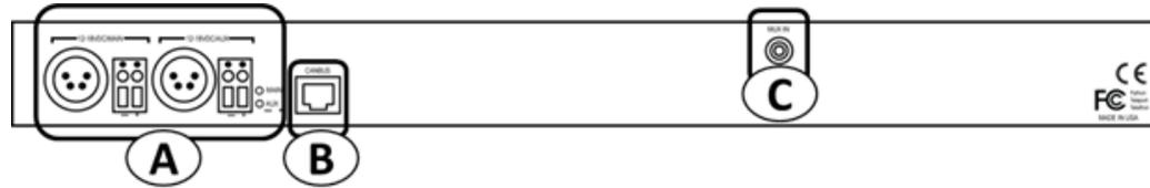
Fig. 3-15: Python 3G Receiver Rear Panel with CWDM
