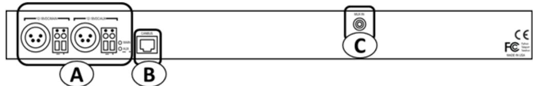
Fig. 3-13: Python 3G Transmitter Rear Panel with CWDM
