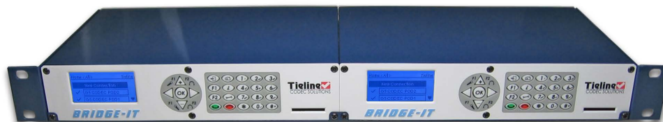
1RU Rack Frame (Optional Accessory) with two Bridge-IT Codecs installed
