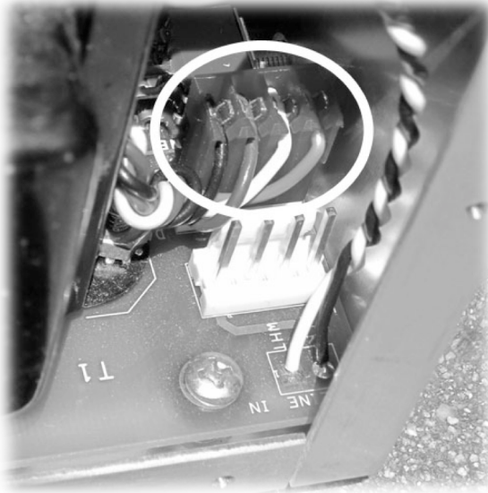
Connector setting for 115VAC input
