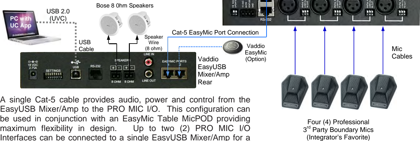
Diagram: PRO MIC I/O 4-Mic Configuration with
