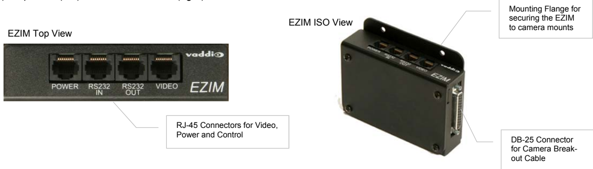
Figure 3: EZCamera Interface Module (EZIM) with four (4) RJ-45 connectors for POWER, RS-232 IN & OUT and VIDEO (HD or SD with IR), Top View (left) and Isometric View (right)
