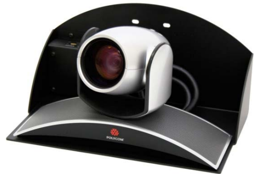
Figure 1: WallVIEW PRO EagleEye System with EagleEye camera, EZIM and Wall Mount (EagleEye camera and Polycom cables are not included).
