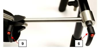
the tilt action of the handles. The same type of lever is used at the shoulder pivot (9). Note that the position of these levers can be adjusted without loosening – simply grab the lever and press on the red button, then you can readjust the angle of the lever without threading or unthreading. This allows you to apply a 'ratcheting action' while tightening or to simply move the lever out of the way without loosening it.
