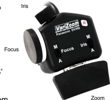
3. **ZOOM CONTROL** - To zoom in (telephoto) press the zoom rocker right, and to zoom out (wide) press the rocker left. The farther you press the rocker, the faster the lens will zoom. The zoom characteristics of the ROCK-PZFI are determined by the camera (e.g., the slowest zoom speed attainable with the DVX100B takes 30 seconds from end-to-end).
