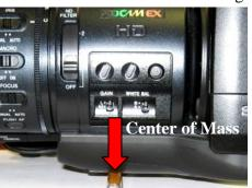
the platform to precisely raise or lower it – you can use a hex key. Try to get the center of mass right on the center of tilt rotation. Rotate the platform to various angles and adjust until it holds position at any angle. If it falls down, you need to adjust the platform upward. If it drifts upward, you need to lower the platform. When balance is achieved, tighten the platform locking lever.
