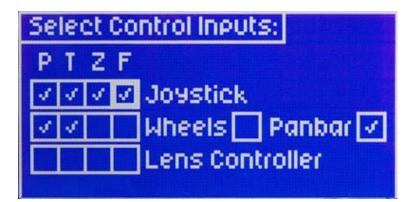
Here is where you can assign how Pan, Tilt, Zoom, and Focus will be controlled. Move the cursor box to where you'd like to control each axis.
