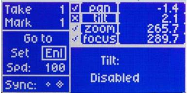
The cursor box then appears in the top right corner, and lets you select one of the four axes. Move the cursor over which axis you wish to control.
