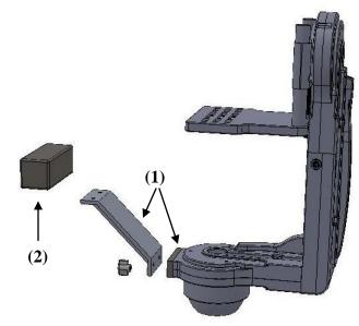
(2) Now attach the square weight to the support arm, using the same type of thumbscrews, lockwashers and washers. Tighten the thumbscrews thoroughly.
