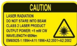
Visible laser radiation. Do not stare into the beam as eye damage may occur. This device contains a class 2 laser. Output power does not exceed 1 mW, wavelength 650 nm.
