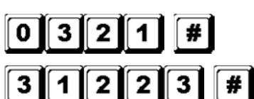
Duress output activates (output switches to ground) and output 1 activates for 1 second
