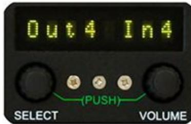
**Out4 In4** - means that AES input #4 will be routed to AES output #4.
