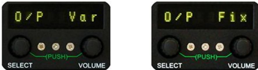
**O/P Var** - means that all the outputs of the unit will be level controlled and follow the action of the VOLUME control
