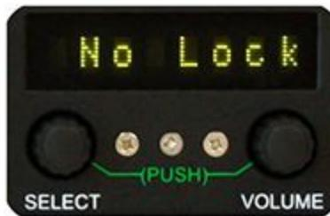
If a signal is present, it will be identified, and the type of signal displayed in the readout window. (There is a slight lag while the processor determines the signal status.)
