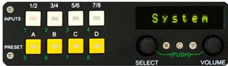
To enter system setup, press and hold INPUT buttons 1/2 and 7/8 with one hand and press the SELECT knob. The readout will display **System**. Press the SELECT button again to enter the mode of operation selection. The readout will display **Mode X**, where X is 1, 2, or 4.
