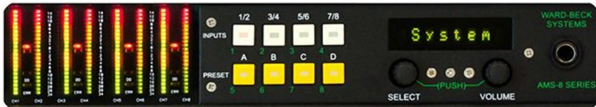
There are eight illuminated push button switches arranged in two rows of four. The upper row designated INPUTS selects the input source to be monitored. The lower row designated PRESETS selects a preset configuration or condition under which the signal is monitored.
