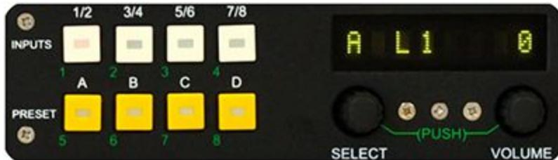
The level can be adjusted for that signal by +/- 15dB by rotating the VOLUME knob clockwise or counter clockwise. The amount of gain or loss from nominal for the selected signal will be displayed above VOLUME knob in a range from **-15** to **+15**.
