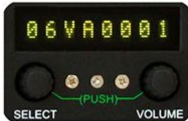
To exit the firmware interrogation mode, rotate the SELECT knob one step counter clockwise and push the SELECT knob once when the readout displays **Exit**.
