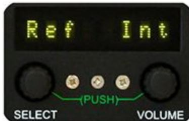
Rotate the SELECT knob another step clockwise to enter the AES OUTPUT #4 Setup. The readout will display **Out4** above the SELECT knob and **In4** or **Mon** above the VOLUME knob.
