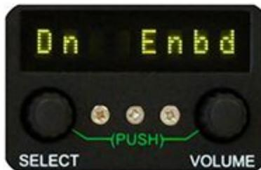
**Dn Enbd** - means that the dialogue normalization level in the metadata will be applied to the dolby signal.
