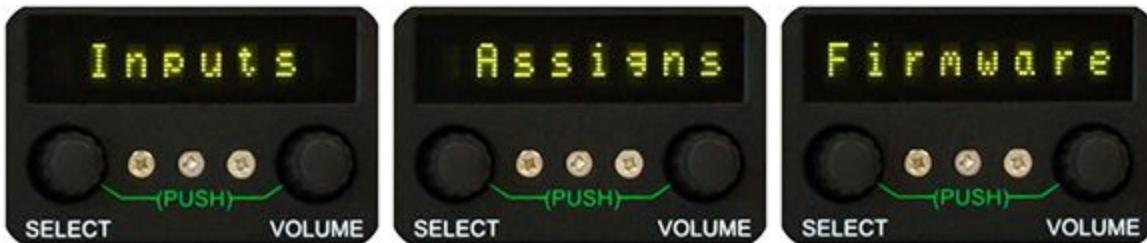
**Inputs** - This configuration setup allows you to select the input sources that will be enabled during monitoring. (See INPUTS SETUP).
