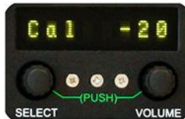
The VOLUME control is used to set the reference level, in two dB steps, for monitoring audio.
