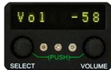
The VOLUME control is used to set the default volume level, in one dB steps, for monitoring audio.
