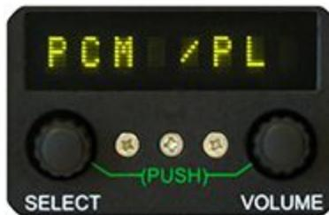
The ProLogic signal comprises Left, Right, Centre, Left rear and Right rear. These signal levels are displayed on the CH1, CH2, CH3, CH5 and CH6 LED bar graphs respectively. To return to the PCM mode, rotate the SELECT knob in either direction.
