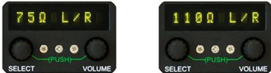
If the unit displays **75Ω L/R**, it means that the bank of four unbalanced inputs is selected. If the unit displays **110Ω L/R**, it means that the bank of balanced inputs is selected. To toggle between the two banks of inputs, press and rotate the SELECT knob.
