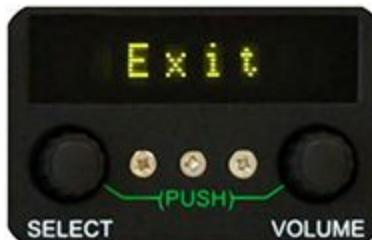
Push the SELECT knob to return to the **System** setup screen. To exit system setup, turn the SELECT knob one step counter clockwise. The readout displays **Exit**. Push the SELECT knob once to exit the system setup procedures.
