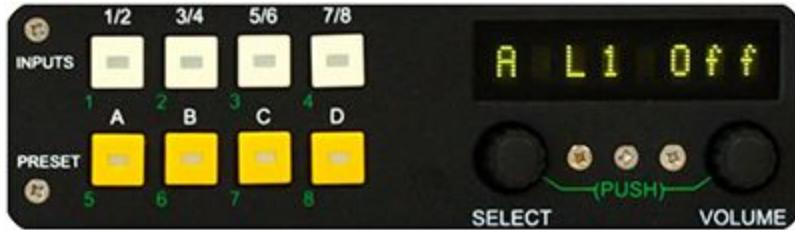
If preset button A is selected, the readout should display **A L1** above the SELECT knob and either **Off** or a level between **-15** and **+15** above the VOLUME knob. Rotating the SELECT knob in either direction cycles through the eight available sources that are displayed on the LED meters.
