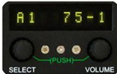
Rotate the VOLUME knob in either direction to select the desired input **75 - 1** to **4**, **110 - 1** to **4**, **ANL -1** to **4**, **SD1 -1** to **8** and **SD2 -1** to **8** to assign **A1**. Rotate the SELECT knob through **A2**, **A3** and **A4** and similarly assign an input source.
