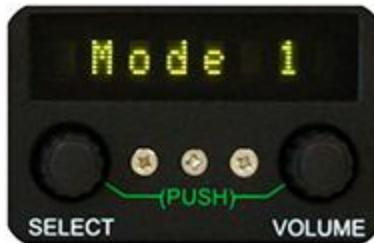
Rotate the SELECT knob one step clockwise to enter the reference signal setup. The readout will display **Ref** above the SELECT knob and **Int, 75Ω** or **110Ω** above the VOLUME knob.
