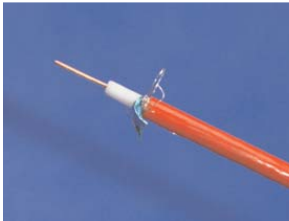
Flair Braid/Shield back over the Jacket. You may have to trim braid/shield to .250"
