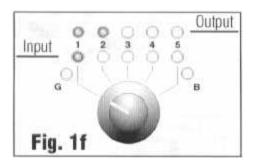
• **SHORT TO GROUND**, the LEDs of the pin being tested will light as well as the Ground LED (Red and indicated with a "G"). If more than one LED lights at the same
