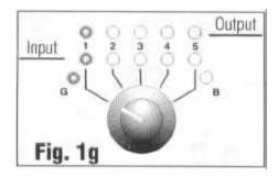
**Note**: In case of the mini (3.5mm) and 1/4" (6.3mm) jack plugs, there are two versions, mono and stereo. When testing mono plugs and the pin selector knob is in position 1 or 3 the LEDs 1 and 3 will light. See Fig. 1h. Notice that in this case the Pin Selector Switch is in positions 1 and 3 respectively.
