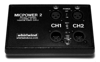
The Whirlwind Micpower 2 (MICP2) is a premium portable stereo phantom power supply. The regulated 48 Volt DC output is ultra quiet, introducing no noise into the microphones' signal path. The Micpower 2 is conveniently portable, operating on four long lasting AA batteries or on AC when desired, by connecting the included PS6V2.5A power supply. The rugged design is perfect for portable recording applications when the use of high quality microphones requires external phantom power.
