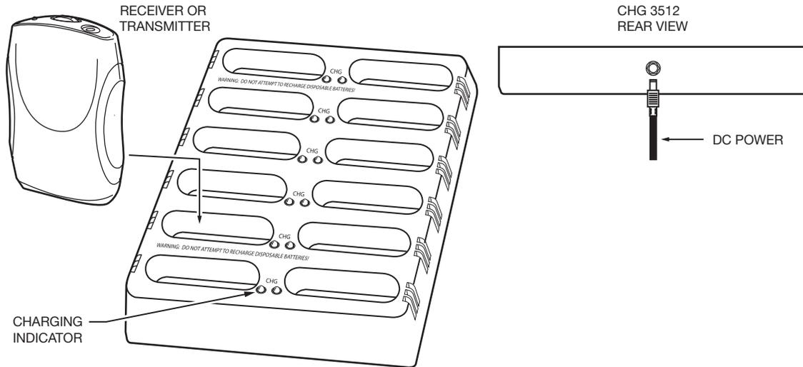
**WARNING: DO NOT ATTEMPT TO CHARGE NON-RECHARGEABLE BATTERIES!** Non-rechargeable batteries, such as alkaline and carbon zinc, may heat up and burst, causing possible injury and damage to the equipment.
