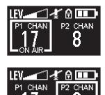
5 . Push the Menu button and note that either "P1" or "P2" shows up on the top left corner of the screen. This indicates which Preset you are adjusting.
