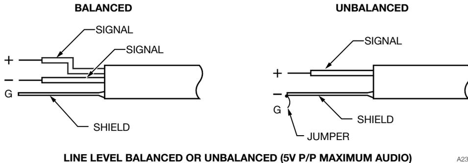
The WIR TX90 will accept line level, balanced or unbalanced audio inputs. If you wish to operate in single channel mode, plug the audio cable with the installed Phoenix connector in “Channel A” OR the “Channel B” connector. If you choose to operate in two channel mode, plug the audio cables with Phoenix connectors in both “Channel A” AND “Channel B” connector.
