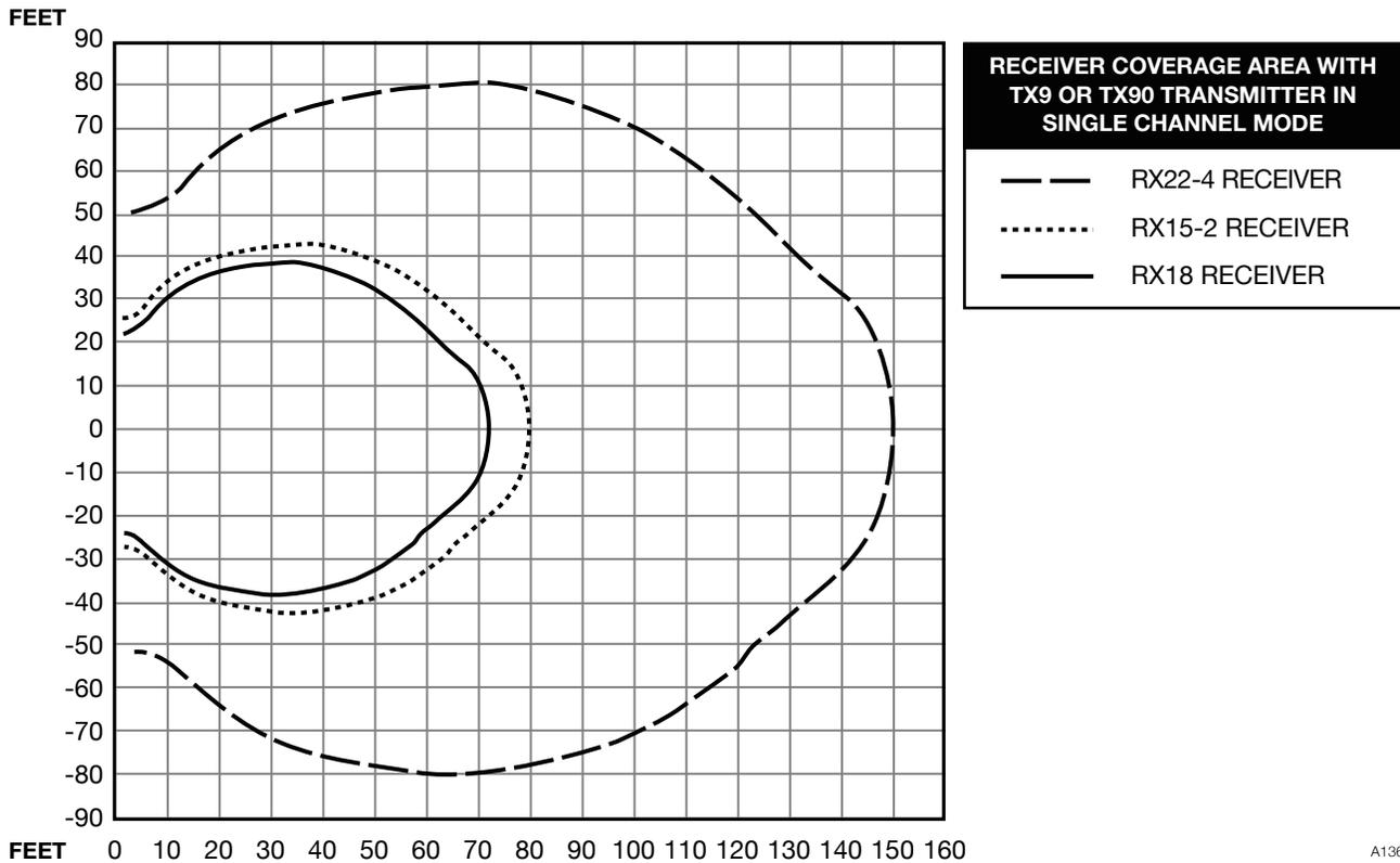
These patterns are the direct radiation pattern. The infrared radiation does not drop to zero outside the illustrated patterns; it decreases. It still may be useable at a greater distance, depending on the receiver sensitivity and the reflective characteristics of the room.
