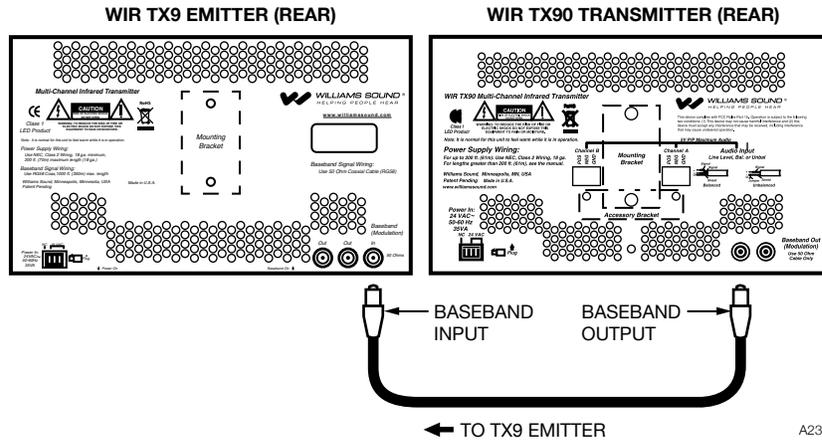
To add a second WIR TX9 emitter panel to the WIR TX90 transmitter, repeat the process above (the WIR TX90 transmitter has two baseband output jacks).
