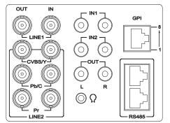
The RMT-173 is designed for a wide range of applications where format flexibility and form factor are key. This monitor is excellent for studio, MCR, Edit suites, ENG & OB production environments. The RMT-173 supports 3G/HD/SD-SDI, HDMI, DVI, composite, Y/C & component video inputs. Featuring a 8-bit 1920 x 1080 TFT/LCD screen and 10-bit image processing, a perfect medium is reached in the scaling and interpolation process, providing superb imaging regardless of video format.
