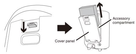
NOTE After the box is removed, loose items, such as the included power cord, speaker cables, owner's manual (this booklet), and an optional microphone can conveniently be stored in the accessory
