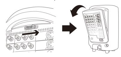
Open the cover panel attached to the other speaker, and then remove the box from inside the accessory compartment.
