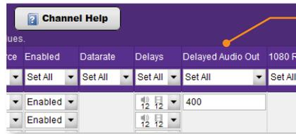
**Delayed Audio Out** found on the Channel Plan tab allows for matching audio to external audio system (first port only).
