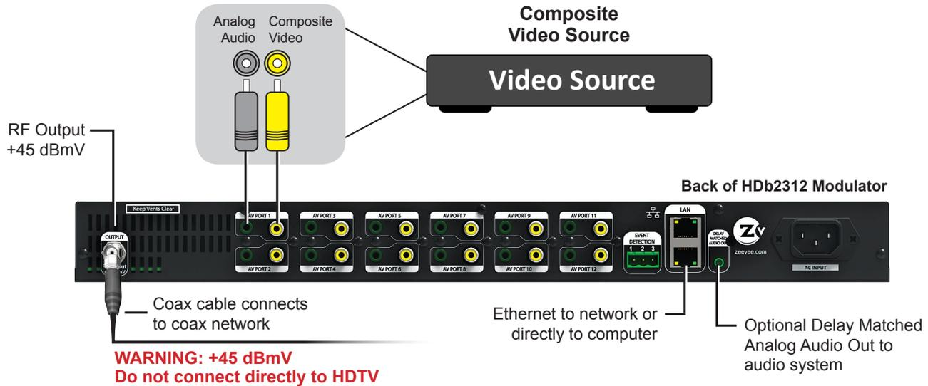
Factory default settings allow HDb2312 series modulators to broadcast up to 12SD sources on RF channels 2, 3, 5, and 6 for reception at connected HDTVs.
