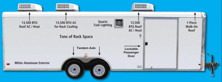
Fully Finished Inside & Out • Dual Suite - 1-Front / 1-Rear • Heat & AC • 6 Racks Console • I/O Panel • Carpeted • Track Lighting • Breaker Panel w/Generator Input
