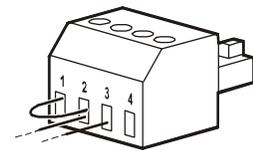
If the contacts are opened, the UPS will turn OFF and power will be removed from the load.
