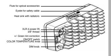
Notes: For mounting, a variety of accessories can be attached using the 3/8" thread on the backside of the LED Panel (see "Grip accessories" on page 19).
