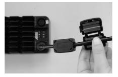
Gently press both sides together to close the suppressor element.
