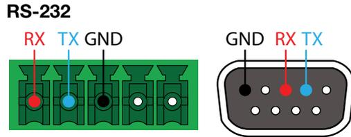
Pin out will be determined by the RS-232 cable and connect as RX (receive), TX (transmit) and  $\perp$  (Ground).
