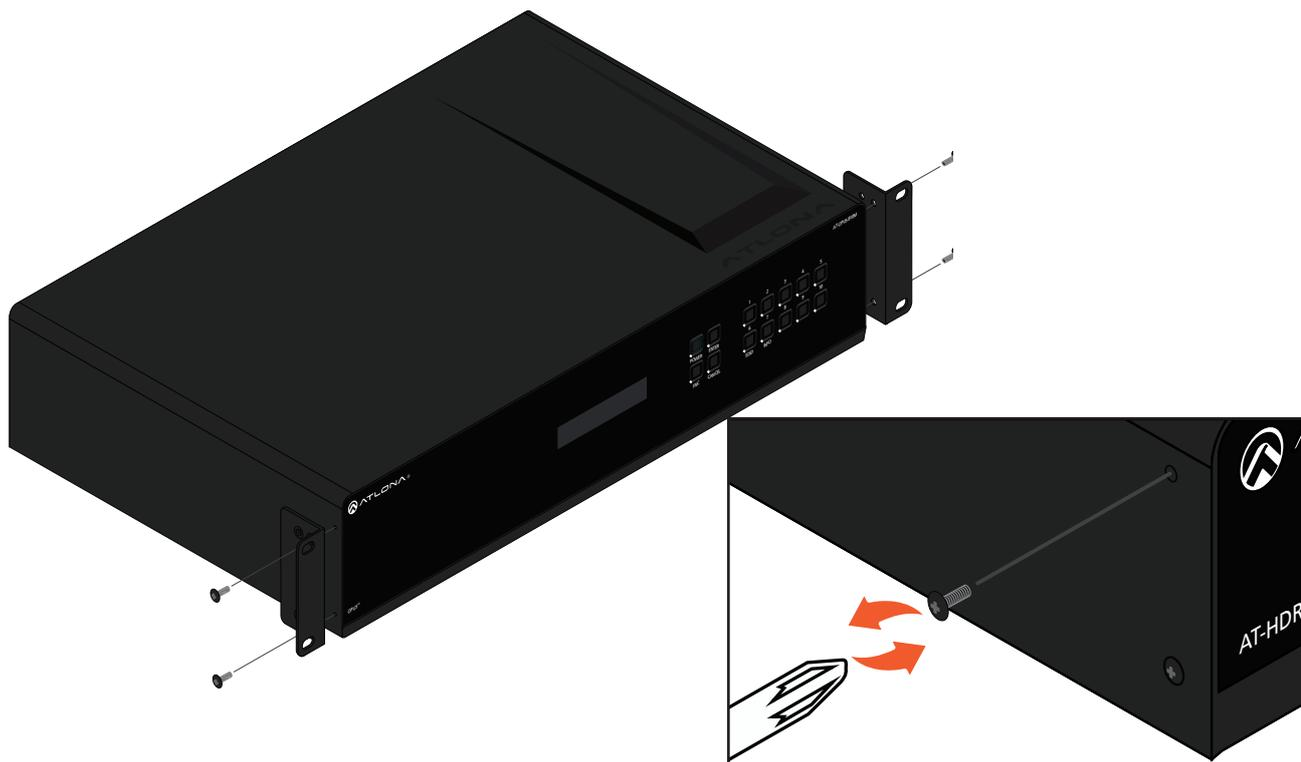
3. Install the Opus matrix into a rack, using four rack screws.
