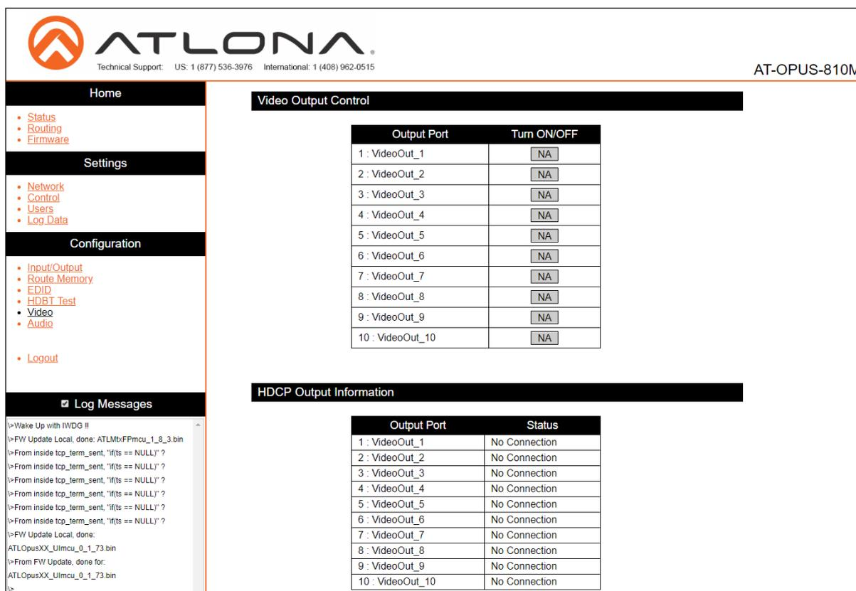
The screenshot shows the AT-OPUS-810M webGUI interface. On the left is a navigation sidebar with sections: Home (Status, Routing, Firmware), Settings (Network, Control, Users, Log Data), Configuration (Input/Output, Route Memory, EDID, HDBT Test, Video, Audio), and Log Messages (checked). The main content area has two sections:
