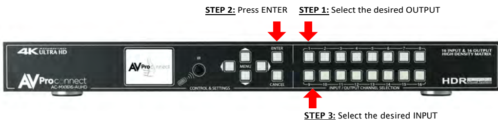
Figure 1 – Switching with the front panel controls. NOTE: Select the OUTPUT and then press ENTER, then select the INPUT
