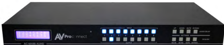
Figure 1 – Switching with the front panel controls. NOTE: Select the OUTPUT and then the INPUT.
