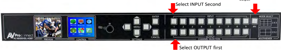
Figure 1 – Switching with the front panel controls. NOTE: Select the OUTPUT and then the INPUT or MV
