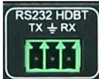
2. **RS232-CTL** - This is for send signals to the AC-SW62-UHD for controlling the device - The Command List can be found on the next page. For convenience there is a notepad version of the Command List on [www.avproconnect.com](http://www.avproconnect.com).
