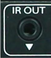
**IR OUT** - The IR OUT port is send IR signals out of an IR Emitter (Pictured below) that originate at the HDBaseT Receiver OR HDBaseT Transmitter
