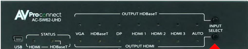
Press and hold this button for 5 seconds to toggle PoE for the HDBaseT **INPUT**. All LEDs will flash if successful.
