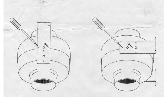
The mounting brackets supplied may be fastened to the in-line fan in either of 2 positions, as illustrated below; use them to mount the fan where most convenient for the particular installation. It may be desirable to use a thin rubber sheet between the bracket and the mounting surface if the surface is a panel which may resonate.
