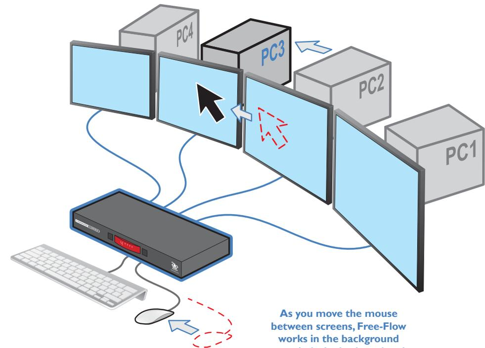
As you move the mouse between screens, Free-Flow works in the background to switch the keyboard and mouse to the corresponding computer.
