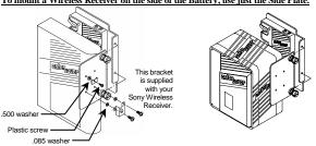
The mounted Sony Audio Clip V Plate mounting uses one (1) 3 x 6 and one (1) .085 washer in top V Plate mounting hole and two (2) 4 x 5 mm pan head and two (2) #6 wahsers in bottom mounting.
