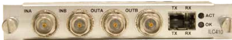
Figure 5. ILC410 BNC Connectors and SFP Socket
