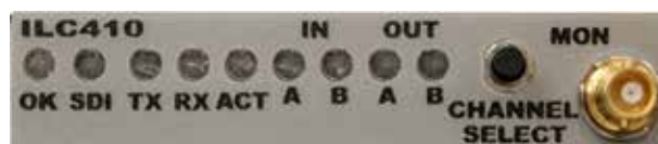
Figure 6. ILC410 Status LEDs and Monitor Connector
