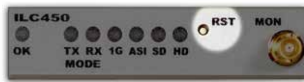
Figure 8. ILC450 Reset Switch
