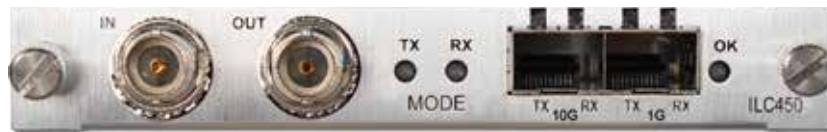
Figure 7. ILC450 Rear Panel Status LEDs
