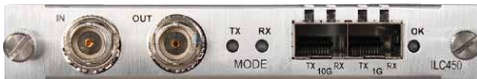
Figure 5. ILC450 BNC Connectors, 10G SFP+ Socket, and 1G SFP Socket
