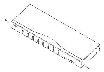
2. Use the M3 x 8 Phillips hex head screws supplied with the rack mounting kit to screw the rack mounting brackets into the sides near the front of the unit.
