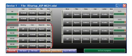
**7.1 Meter** – There are four bar graph meters that illustrates the level of the output signal of the generator, it is POST the channels gain control and PRE input filters.
