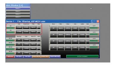
**6.1 Input Meter -** The bar graph meter illustrates the level of the input signal POST the channels gain control and is PRE input filters and compressor settings.
