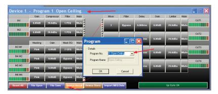
**9.5 Device Store** - The ASP-MG24 has a built in non-volatile memory that can store up to 30 different program setups. A program can be stored using this menu. The old program with the same program number will be replaced. Once the program is stored in the flash memory, it can be recalled at a later time, even after power down.
