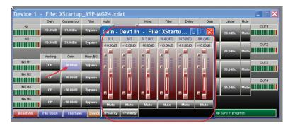
**7.6 Masking EQ** - When clicking on the filter screen, 3 sub viewing screens appear. Note: All three screens can be moved for personal viewing preferences.
