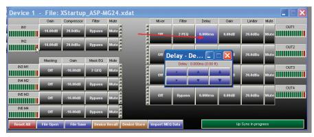
**8.7 Gain** - The four output gain levels are shown when clicking on this window. Controlling the gain can be accomplished by dragging the fader or by using the up down buttons or by typing in number viewing text box. Channel Mute can be accomplished by clicking on the Mute tab and will illumination Red indicating the channel is in Mute. Input Polarity can be set by clicking on the tab.
