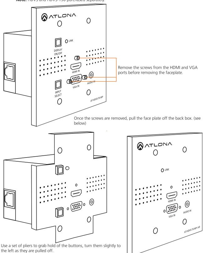
Once the buttons are removed, place the AT-HDVS-TX-WP-NB on the front of the HDVS wall plate and replace the screws. Installation is complete and the HDVS is ready to be used again.
